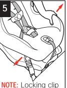
With weakest hand at belt path, tilt and push the child restraint forward and back, and from side to side. If the seat belts do not loosen, your child restraint should be secure.
